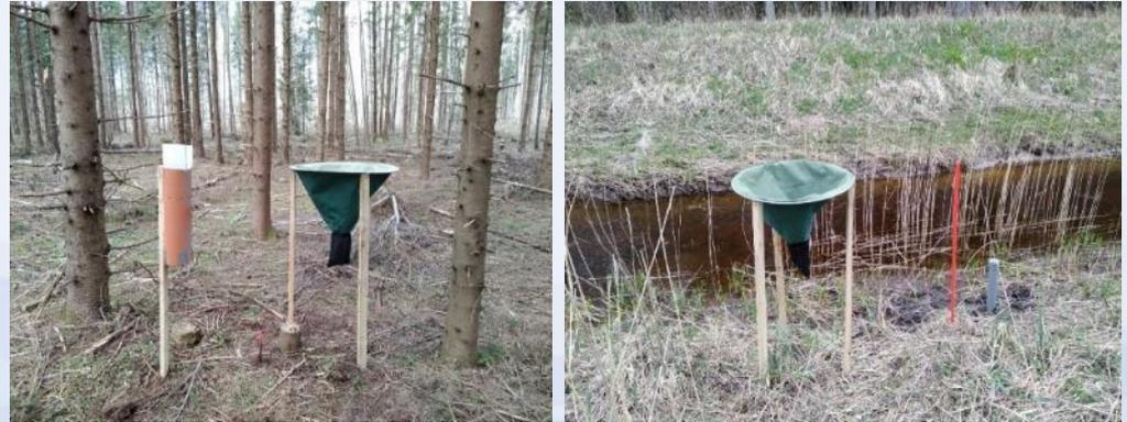
*Planned measures (above), example of monitoring points along Age tributary Tora (left) and monitoring equipment – precipitation, litter and groundwater samplers*
