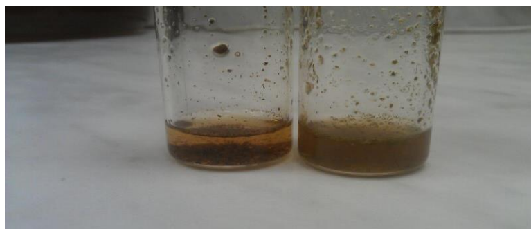
Figure 2.6: Growth of microorganisms in hydrolisates from untreated substrates (right) as opposed to heat treated substrates (left)
