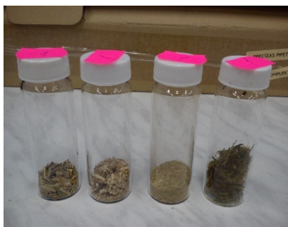
Determination of most appropriate biomass fraction size for enzyme hydrolysis
