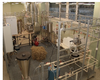
Biobutanol production pilot facility
