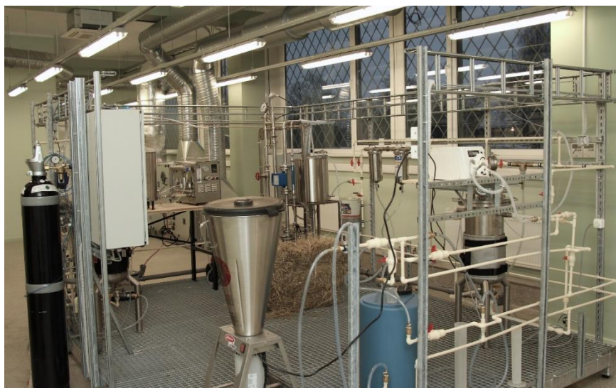
Figure 8: Biobutanol production pilot located at Riga Technical University (constructed in 2013)
