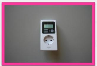
This measuring tool is easy to use - electrical plug of your household device has to be plugged into the socket of the measuring device and the plug of the meter — into the electrical socket. Depending on the manufacturer the price of the measuring tool vary in a range from 10 to 30 EUR.
