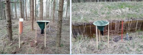
*Planned measures (above), example of monitoring points along Age tributary Tora (left) and monitoring equipment – precipitation, litter and groundwater samplers*
